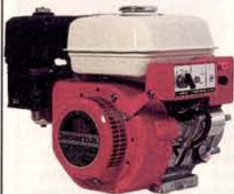
GX140- a 5HP* OHV horizontal-shaft engine (144cm 3 ) with electronic ignition and Oil Alert. Suitable for powering air compressors, generators, pumps, pressure washers, reel-type lawn mowers, and other construction equipment.
