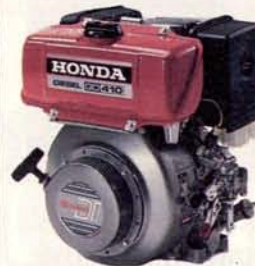
SPECIFICATIONS GD410- Rated Output (HP/RPM): 8/3,600 Max torque (kgm/RPM): 2.1/2,500 Fuel Capacity (l): 4.6 Oil Capacity (l): 1.25 Dry Weight (kg): 54 (LxWxH-mm) 440x405x490 Fuel g/HP-Hr: 178
