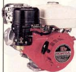
GX110- a 3.5HP* OHV horizontal-shaft light-weight engine (107cm 3 ). Includes Automatic Decompression and Oil Alert suitable for edgers, pumps, small construction equipment and reel-type mowers.
