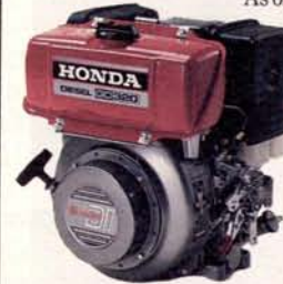
SPECIFICATIONS GD320- Rated Output (HP/RPM): 6/3,600 Max torque (kgm/RPM): 1.6/2,500 Fuel Capacity (l): 4.6 Oil Capacity (l): 1.15 Dry Weight (kg): 48 (LxWxH-mm) 420x405x470 Fuel g/HP-Hr: 180
