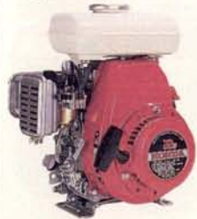
G100- a 2.2HP* horizontal-shaft side valve light-weight engine (83cm 3 ). Includes Automatic Decompression, mechanical governor and electronic ignition, suitable for edgers, pumps and small mowers.
