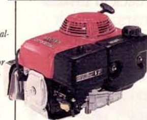
GXV340- an 11HP* OHV vertical-shaft engine (337cm 3 ) with easy-maintenance features, Oil Alert, and electronic ignition. Suitable for powering slashers, turf equipment and ride on mowers.
