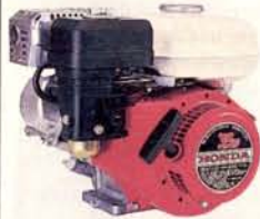
GX110- a 3.5HP* OHV horizontal-shaft light-weight engine (107cm 3 ). Includes Automatic Decompression and Oil Alert suitable for edgers, pumps, small construction equipment and reel-type mowers.
